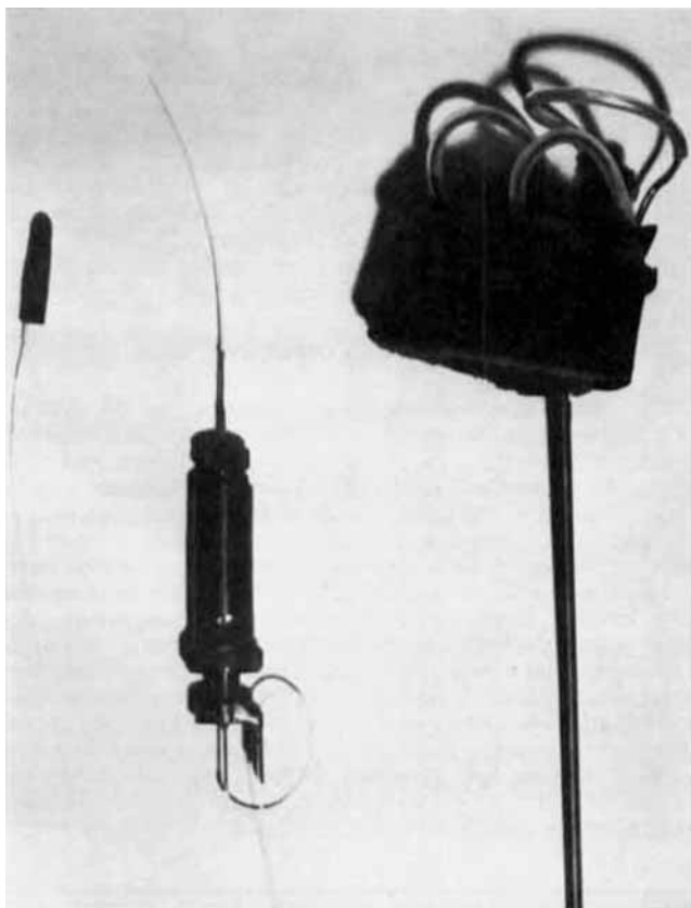
Figure 1 —Photograph displaying gastric motility recording apparatus. From left to right: intragastric balloon with polyethylene inflation tube, fluid swivel assembly, and spring-guide and harness.
